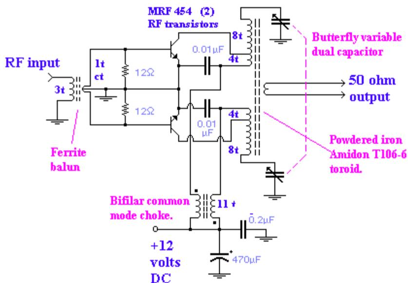
Amplifier # 1. **A simple class B tuned amplifier.** This works, but I don't recommend it.
