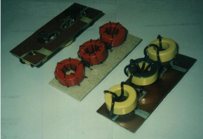
Chebyshev output low pass filters for an untuned class B. They plug into a card edge connector.
