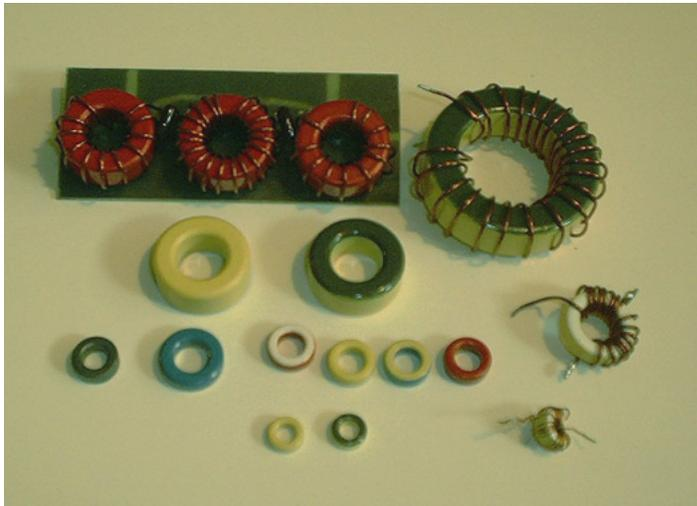
**First:** Select the type and size of toroid core appropriate for the frequency and power level. There are several grades of powdered iron and ferrite cores that are designed for different frequency ranges. For resonant circuits or filters on the upper HF hambands, I usually *use type 6 powdered iron (color code yellow and black)*. For the lowest
